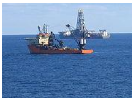
Fig. 2: The Drillship Discoverer Enterprise is shown in the background, at work during exploratory phase of a new offshore field. The Offshore Support Vessel Toisa Perseus is shown in the foreground, illustrating part of the complex logistics of offshore oil and gas exploration and production. (Source: http://www.wikipedia.org )
