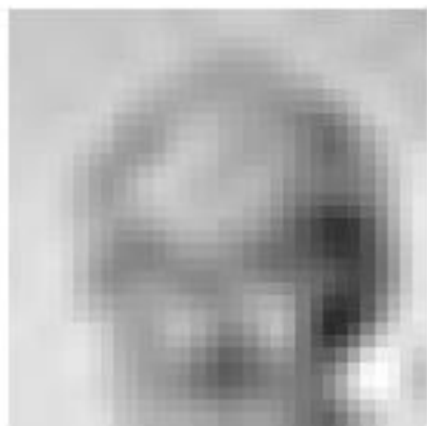
Fig. 3.4: 32 \times 32 Pixel Image Reconstructed from 10 \times 10 Subset of DCT Coefficients. Overall information has been retained, but some detail has been lost
