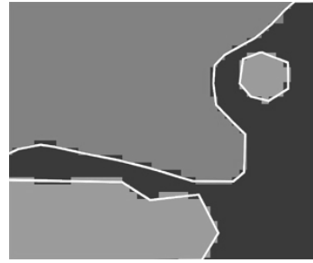
Fig. 4.7b: Magnified Views of the Same GIS Data File Converted into Vector Format
